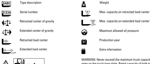
WARNING: Never exceed the maximum truck capacity as seen on the truck type plate. Rated capacity of both truck and attachment is the responsability of the original truck manufacturer and may be less then the capacity shown on the attachments type plate.
